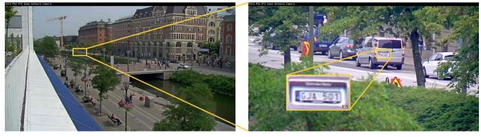
Images from AXIS P54. Left: wide view. Right: 18x zoomed-in view where the license plate of a vehicle 200 m (660 ft) away can be read.
