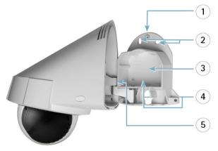
An AXIS P54 camera comes with a built-in wall bracket (1) for easy installation. Oblong screw holes (2) make leveling easier. Extra space (3) is provided for service loops and there are holes (4) for cables. With a lift-off hinge (5), the camera, together with the integrated sunshield, is easily hung onto the wall bracket, freeing up hands to make cable connections. The hinge allows the camera unit to swing in and be fastened
