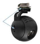
An AXIS P54 camera is directly attached to the drive shaft of two motors (pointed out in image at left)—one for panning and another for tilting the camera. With no parts such as belts or gears, AXIS P54's durable pan/tilt system is fast and provides customers with a reliable, low-maintenance PTZ camera.
