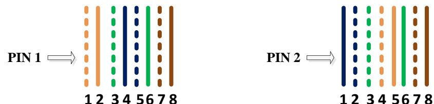
3. Put the wires into two PINs of RJ—48 joint according to the abovementioned sequence of the wires.
