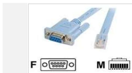
**Step 2:** Connect the F port of the serial cable to the COM port of PC.
