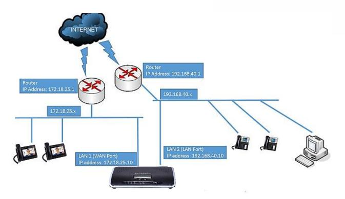
Figure 13: UCM6202 Network Interface Method: Dual
