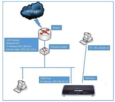
Figure 12: UCM6202 Network Interface Method: Switch
