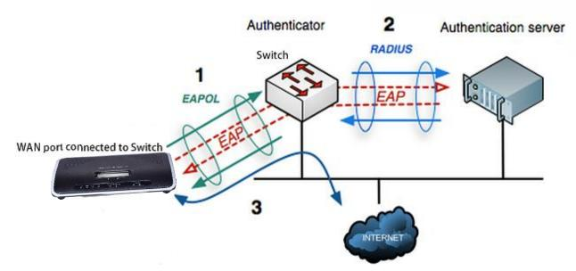
Figure 17: UCM6200 Using 802.1X as Client
