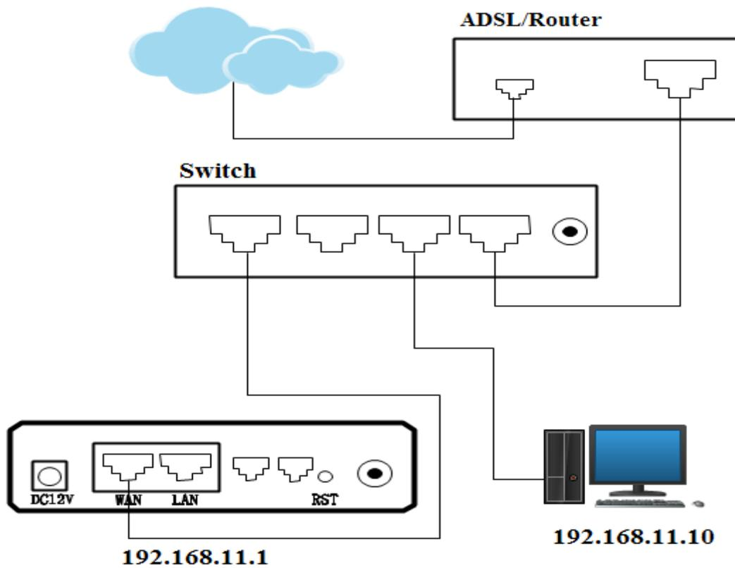
Note: The IP address of PC and the IP address of WAN port of UC100 are at the same network segment.
