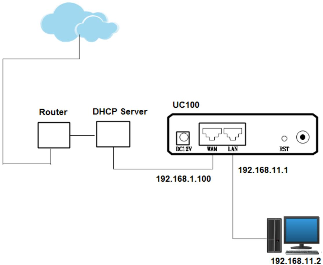
Note: The IP address of LAN port of UC100 and the IP address of PC are at the same network segment, while the IP address of WAN port is at a different network segment.
