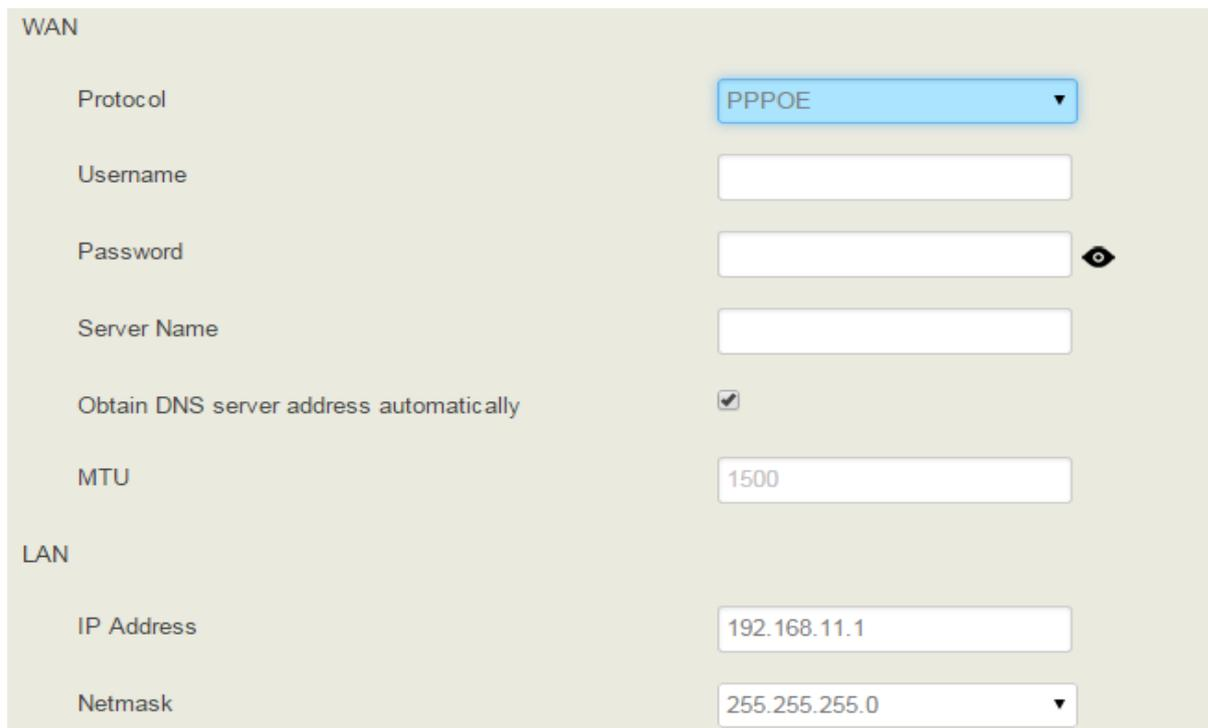
The screenshot shows a configuration interface for WAN settings. The 'WAN' section is highlighted. The 'Protocol' is set to 'PPPOE'. The 'Username' and 'Password' fields are empty, with a toggle icon for the password. The 'Server Name' field is empty. The 'Obtain DNS server address automatically' checkbox is checked. The 'MTU' is set to 1500. The 'LAN' section is also visible, with 'IP Address' set to 192.168.11.1 and 'Netmask' set to 255.255.255.0.
